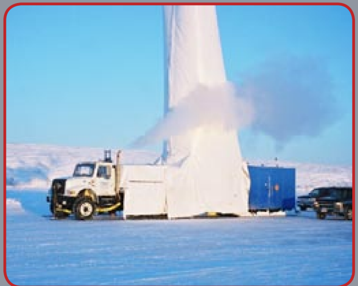
■ Drilling for the placement of seismic explosives for oil and gas exploration.
