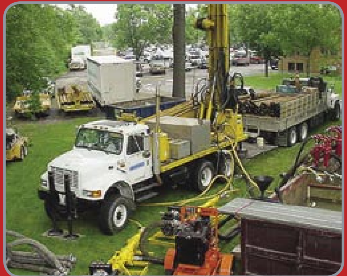
■ Preparation for large diameter multi-cased deep environmental exploration in artesian conditions.
